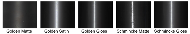
Fig. 6. Photos of our printed varnishes on a cylindrical setup with a line light source.
